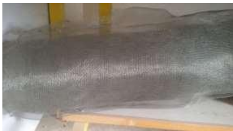
(a) reinforcing wire mesh type 1
