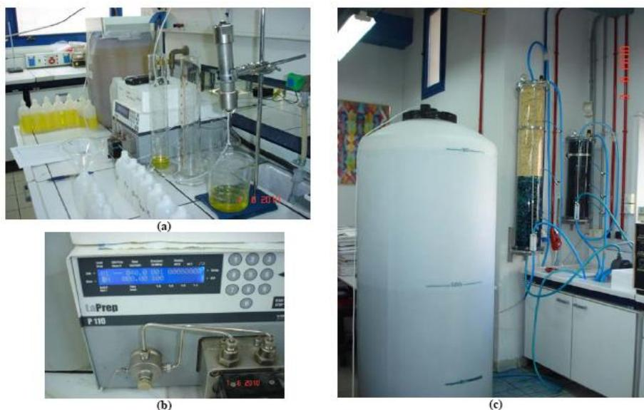
Figure 2. (a) Laboratory scale column of 15 cm height with 25 L tank, (b) laboratory scale pump, and (c) pilot scale column of 137 cm height with 1000 L tank.
