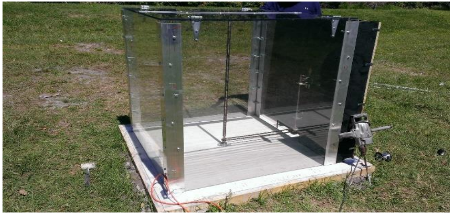
Figure 3 Housing Unit with lifting mechanism
